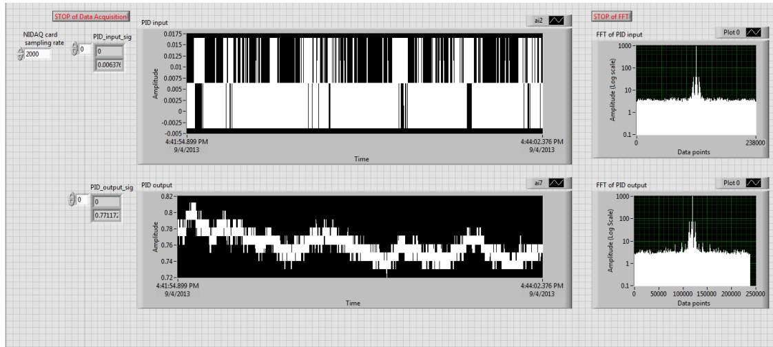
Figure 2.11: 1083 nm diode laser SAS locking signal.
