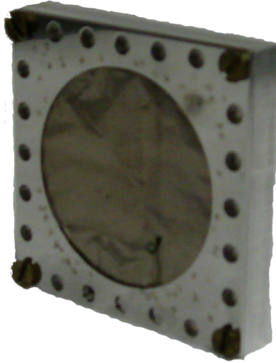
Figure 4.10: Sample mount used to expose boxes early in the experiment
