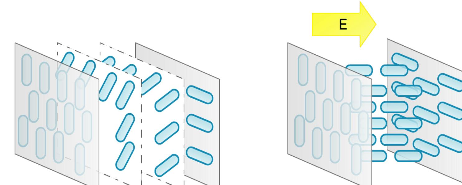
The SDE1024 is a liquid crystal on silicon [LCoS] SLM. LCoS is always reflective. Incident light travels through the liquid crystal cell and reflects off the back silicon wall.
