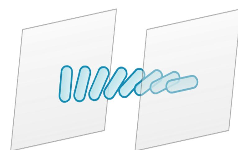
The front and rear surfaces of the SLM cells are electrically conducting and are coated with thin alignment layers that are rubbed to establish a preferred orientation for the nematic molecules.
