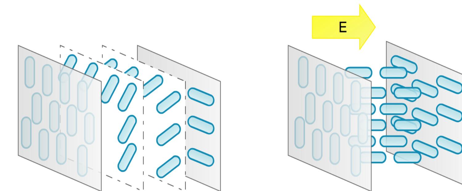
The SDE1024 is a liquid crystal on silicon [LCoS] SLM. LCoS is always reflective. Incident light travels through the liquid crystal cell and reflects off the back silicon wall. When this reflection occurs, the polarization axis of the light will be shifted  $180^\circ$ . In the case of twisted nematic SLM's, this shift will cause the incoming and outgoing polarization of the light to be the same with no voltage applied.
