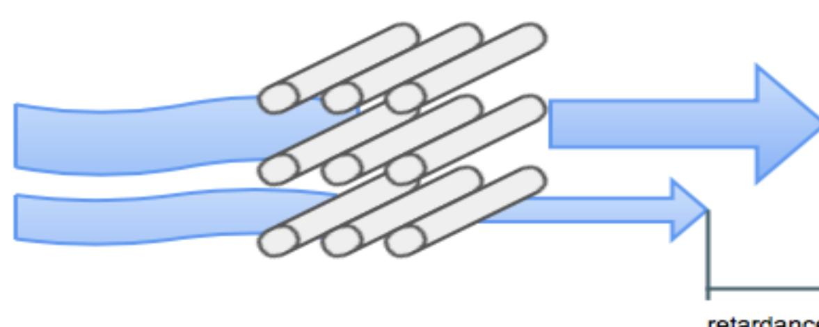
Liquid crystals can exist in a variety of configurations. One such liquid mode is *twisted nematic*. Liquid crystals are twisted nematic when the molecules are twisted into a helix with long axis of the front-most and back-most molecule usually being perpendicular. Because light is scattered along the axes of the molecules, the incident polarization follows the rotation of the helix.
