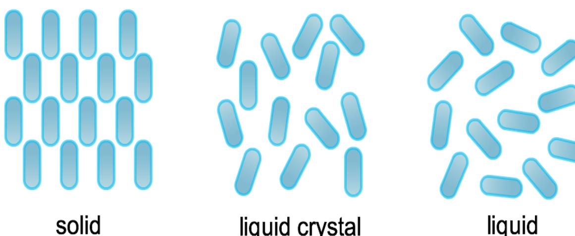
They are birefringent meaning different polarizations of light can experience different indices of refraction.
