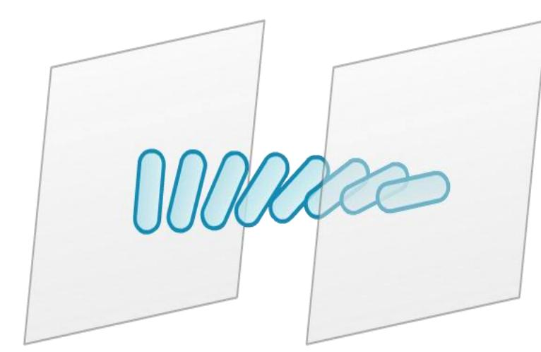
Our SLMs are electrically-addressed. This means that we can modify the properties of liquid crystals pixels by applying a voltage signal to the SLM.
