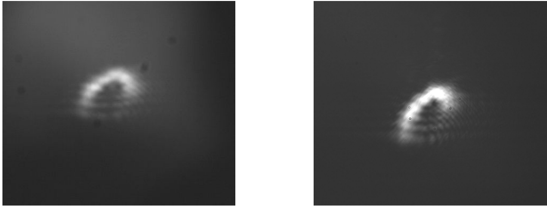
Figure 19: Cut mode imaged at 10 cm and 14 cm from the straight edge.
