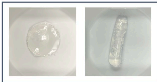
Figure 1: 20% PVA-MA UV crosslinked with Irgacure 651. 3D disk (left), 3D tube (right).
